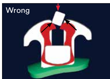
Wrong If the wire does not enter the clip correctly, it can create a positive stop (black arrows) and resist easy wire insertion.
