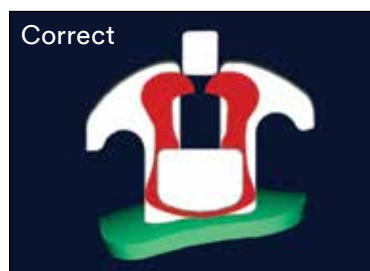
Correct Insert wire perpendicular to the base of the slot. This may require torquing of the wire.
